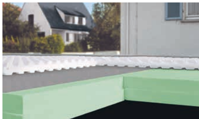
Fig. 22: Styropor compact boards for the retention and drainage of water on a green inverted roof with Styrodur®.
