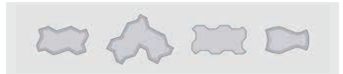
Fig. 46: Stone shapes for stable pavement.
